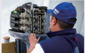
One of the practical tests involved disassembling and re-assembling the camshaft of an F225A
